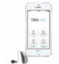
Starkey's Halo hearing aid was one of the first made-for-iPhone hearing aids to come on the market. Its TruLink app enables users to perform a variety of functions using an iPhone.
